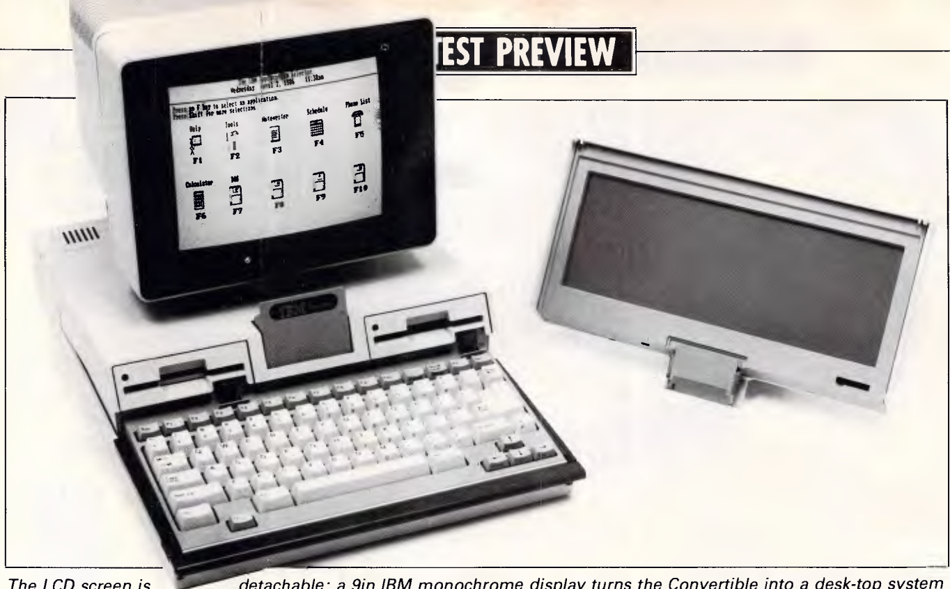
The LCD screen is detachable; a 9in IBM monochrome display turns the Convertible into a desk-top system
